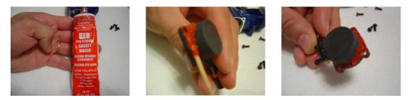
Once the Back Plate is clean and dry, carefully spread red silicon sealer (Wal-Mart and auto parts stores) around the seal of the back plate.
