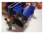
Before you mount the engine, unscrew and remove the back plate using a number 1 Phillips screwdriver. Push hard on the screws so that the heads don't strip. Optionally you can replace the back plate screws with M2.5 x 8 socket head machine bolts, but this isn't necessary.
